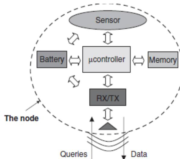
Figure 2: Architecture of sensor node
